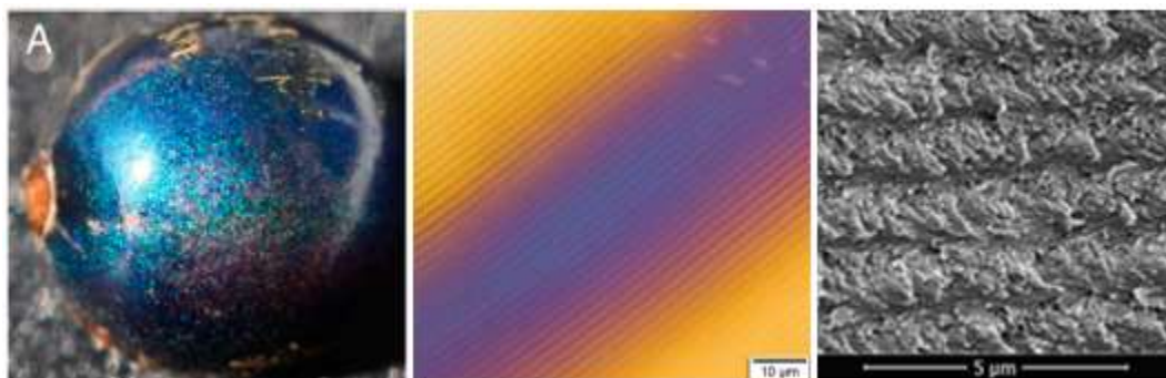
Figure 1: a) Pixelated rainbow-like aspect of Pollia Condensata 1 . b) « Fingerprint pattern » of cholesteric cellulose nanocrystals in polarized optical microscopy. c) Cholesteric helices observed in scanning electron microscopy.
