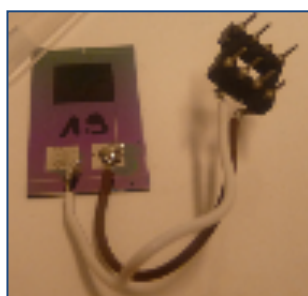
Image of a polypyrrole-based gas sensor
